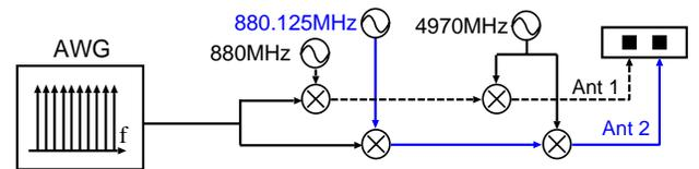
Figure 3. Transmitter block diagram.
