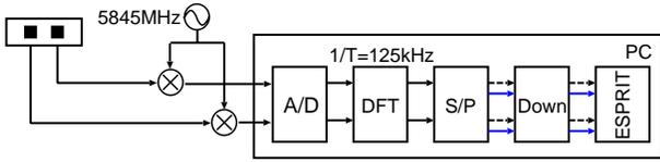
Figure 4. Receiver block diagram.
