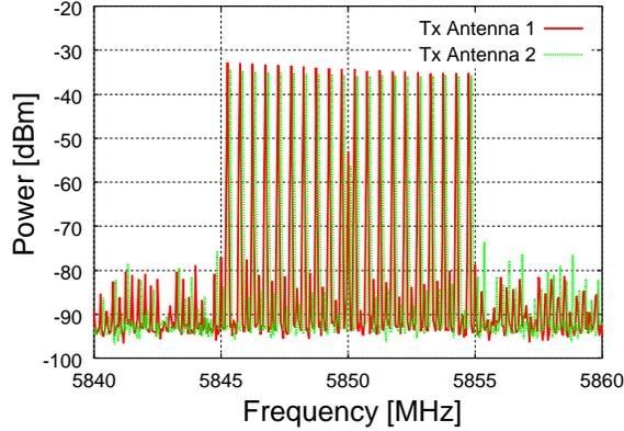
Figure 5. The spectrum of transmitting signals.
