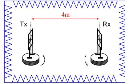
Figure 6. Measurement setup in the anechoic chamber.
