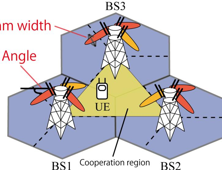
**Base station antenna directivity is required to be designed differently from conventional way**
