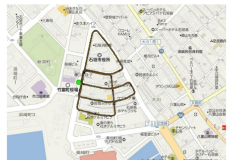
Fig : Measurement area: urban microcell environment in Ishigaki, Japan at 11 GHz band
