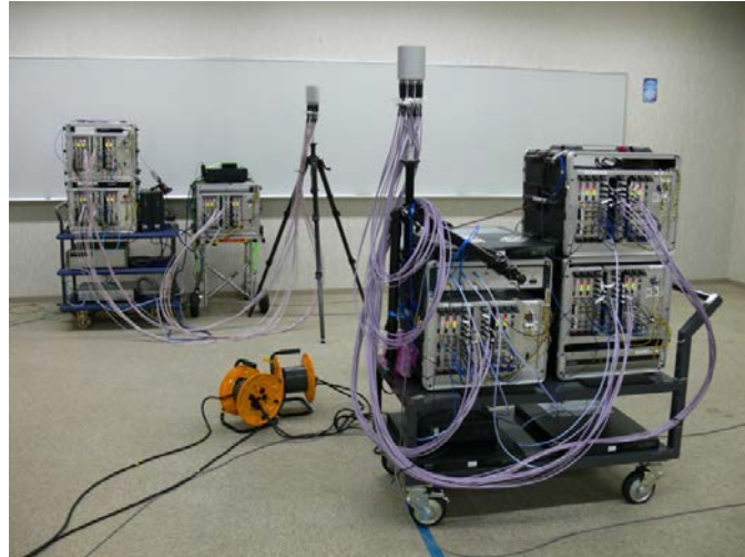
Fig. 4. Double directional channel measurement in 24 \times 24 MIMO configuration
