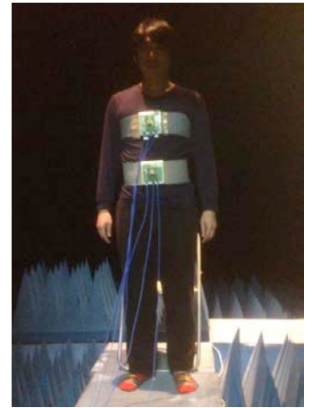
Fig. 10. BAN channel measurement example: chest-navel link
