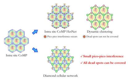
Fig4. Conventional cellular network and Diamond cellular network
