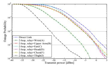
Fig.14 (Left) UWB Measurement System. (Right) Outage probability of ankle-navel link compared with two-hop links in 2.4GHz BAN while walking.
