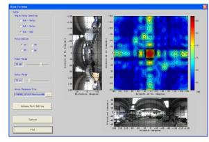
Fig. 5 The GUI of the in-situ validation tool. The measured data is analyzed and converted to angle-delay power spectrum that can be compared with the panorama pictures
