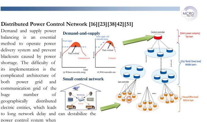
Fig.27 Hierarchical Distributed Control Network
