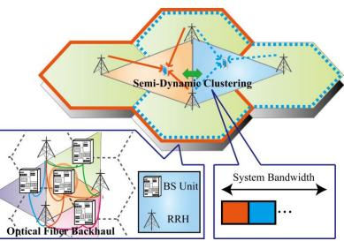
Fig. 1 Shared Remote Radio Head Architecture
