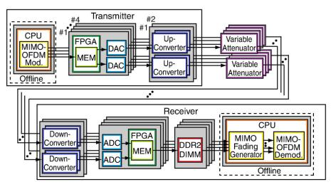
Fig. 14. 11 GHz band 8x8 MIMO-OFDM experimental system
