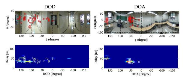
Fig. 2 Indoor double directional measurement example; results of beamforming and SAGE (space-alternating generalized expectation-maximization)
