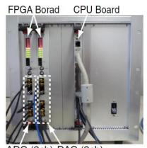
ADC (2ch) DAC (2ch) Fig. 12. 60 GHz transceiver of OFDM experimental system
