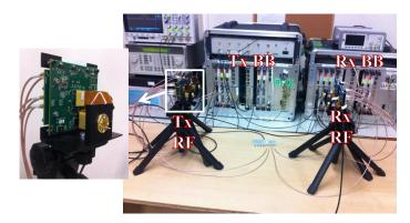
Fig. 6 60-GHz Millimeter-wave Channel Sounder
