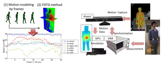
Fig. 13 (a) FDTD Simulation procedure and obtained result of link fluctuation (b) Integrated simulation and measurement environment using Kinect
