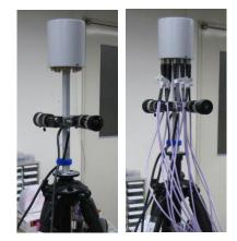
Fig. 3 The assembly of fisheye cameras and circular array antenna (Left: w/o RF cable. Right: with RF cables).
