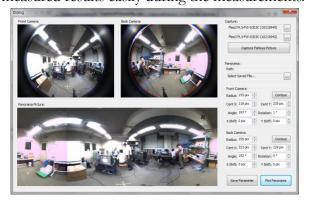
Fig. 4 The GUI of camera selection and setting, in where the upper two pictures are taken with the fisheye cameras and the lower picture is the panorama combined from the upper two fisheye pictures.
