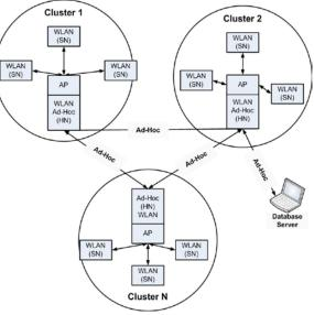
Fig.10 Cluster based Sensor Networks
