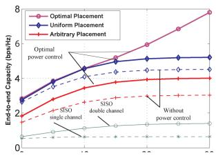
End-to-end capacity vs. Max Tx. Power
