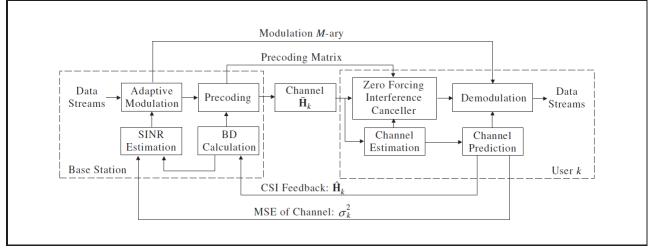
System design for robust multiuser block-diagonalization
