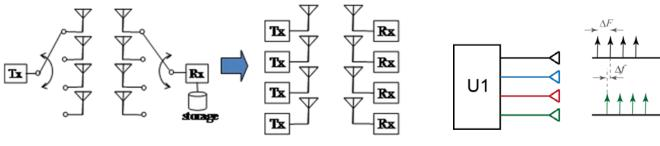
Fig.6 MIMO Channel Sounder Structure
