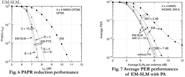
To evaluate the influence of the nonlinear distortion, PER performances of EM-SLM with 64QAM were investigated. The results are shown in **Fig. 7**. It can be seen that with the input backoff (IBO) = 5 dB, the normal EM suffers from the nonlinear distortion by power amplifier (PA), while EM-SLM with U = 16 can limit  $E_b/N_0$  degradation at PER = $10^{-2}$  to 0.9 dB, and it can gain 2.7 dB in comparison with EM by the PAPR reduction effect.
