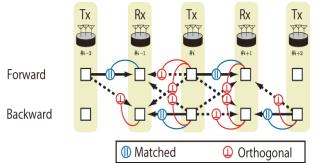
Inter-stream interference is eliminated by Tx/Rx weight control, which results in high spectral efficiency.
