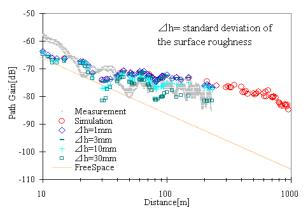
compared with measurements made inside an arched tunnel. Fig.15 Path gain results with the rough surface. Next, the effect of rough surface is introduced in the ray tracing simulation, and simulation results are compared with measurement data.
