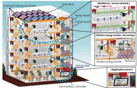
Building control system by wireless grid Prototype Hardware for Wireless Smart Grid [15, 37-39]
