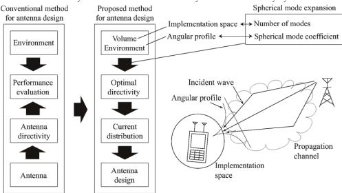
Spherical Mode Expansion - based diversity antenna design
