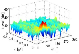
Fig.18 Received Signal Dispersed in Delay and Azimuth
