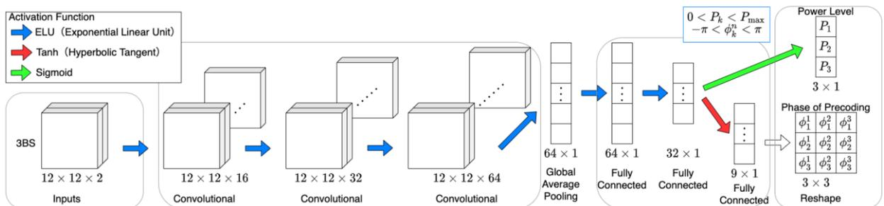
Fig. 2. The structure of CNN.
