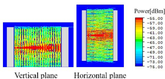
Fig. 1 Power Distribution by an Array Antenna Beam
