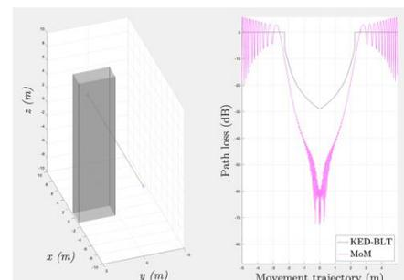
Fig. 2 preliminary result and validation in 2D
