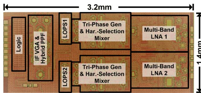
Fig. 6. Block diagram of proposed multi-band phased-array receiver.
