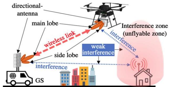
Fig. 6. Spectrum sharing with terrestrial systems
