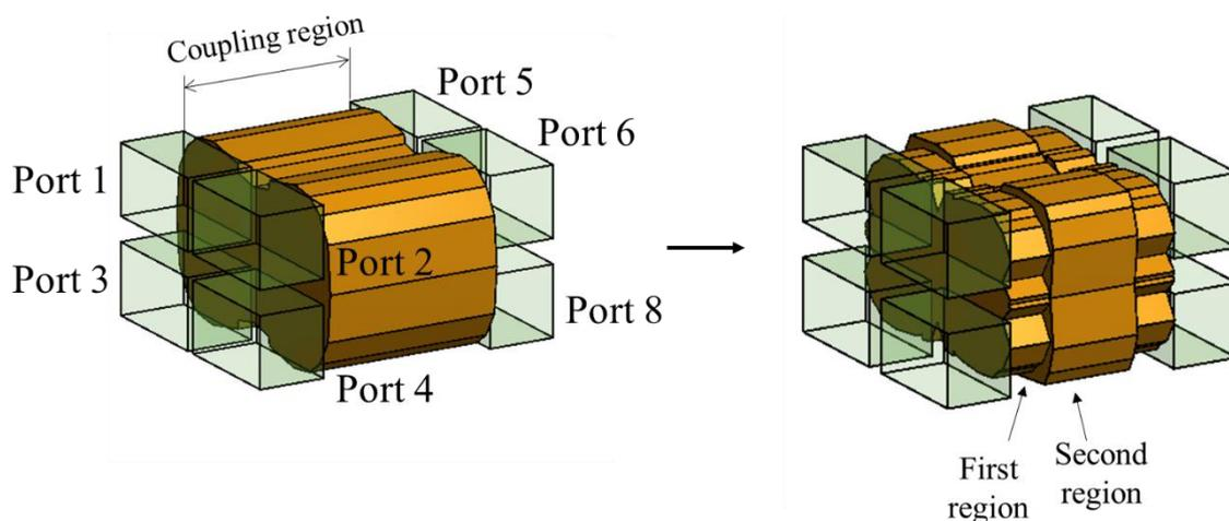
Fig1. Comparison of conventional and new model of two-plane hybrid coupler
