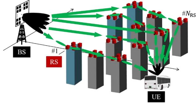
Fig. 3: Massive Relay SU-MIMO System
