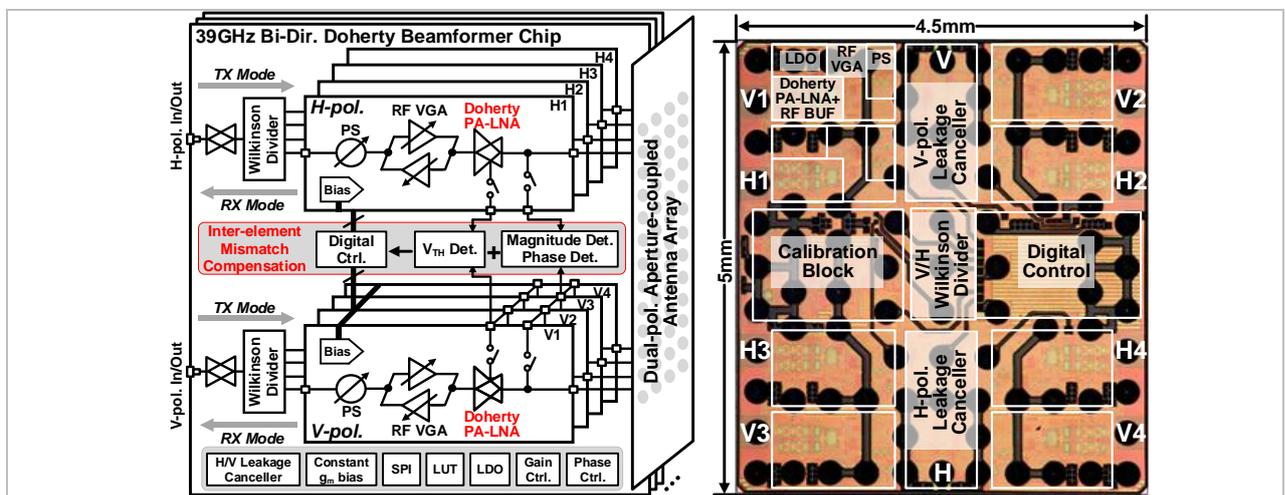
Fig. 1. Proposed 39GHz phased-array transceiver with inter-element mismatch comp. technique.
