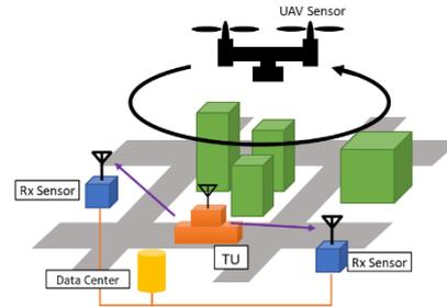
**Fig. 12 Localization using UAV sensor**
