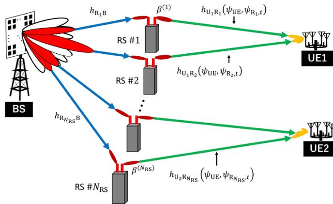
Fig. 4: Massive Relay MU-MIMO System
