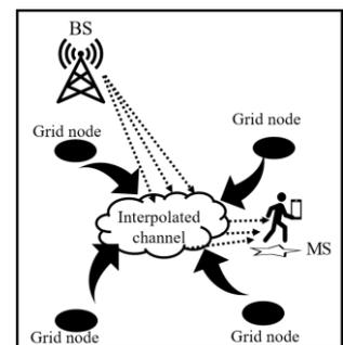
Figure 1 channel emulation architecture
