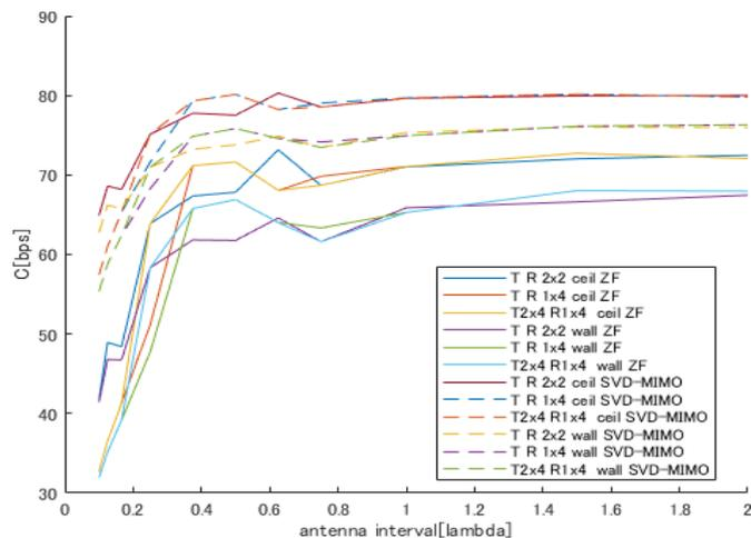
**Fig. 15. Comparison of antenna spacing of dipole antennas and communication capacity for each coding method**
