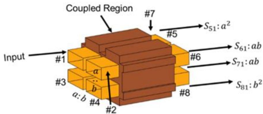
Fig. 1 One body two-plane coupler with nonuniform division
