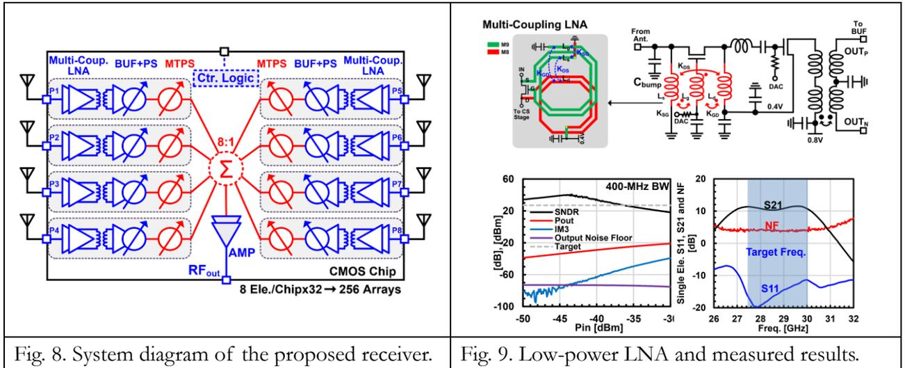
Fig. 8. System diagram of the proposed receiver.
