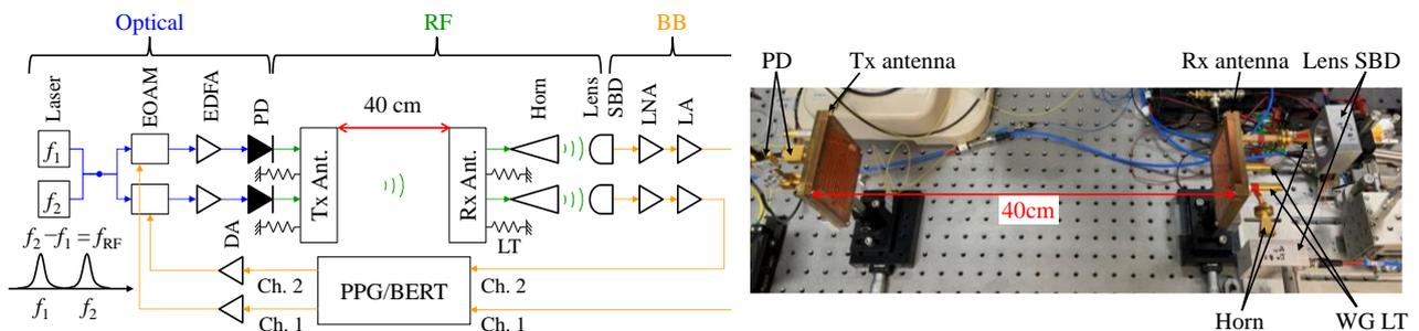
Fig. 1 Wireless Transmission Test Configuration [4]
