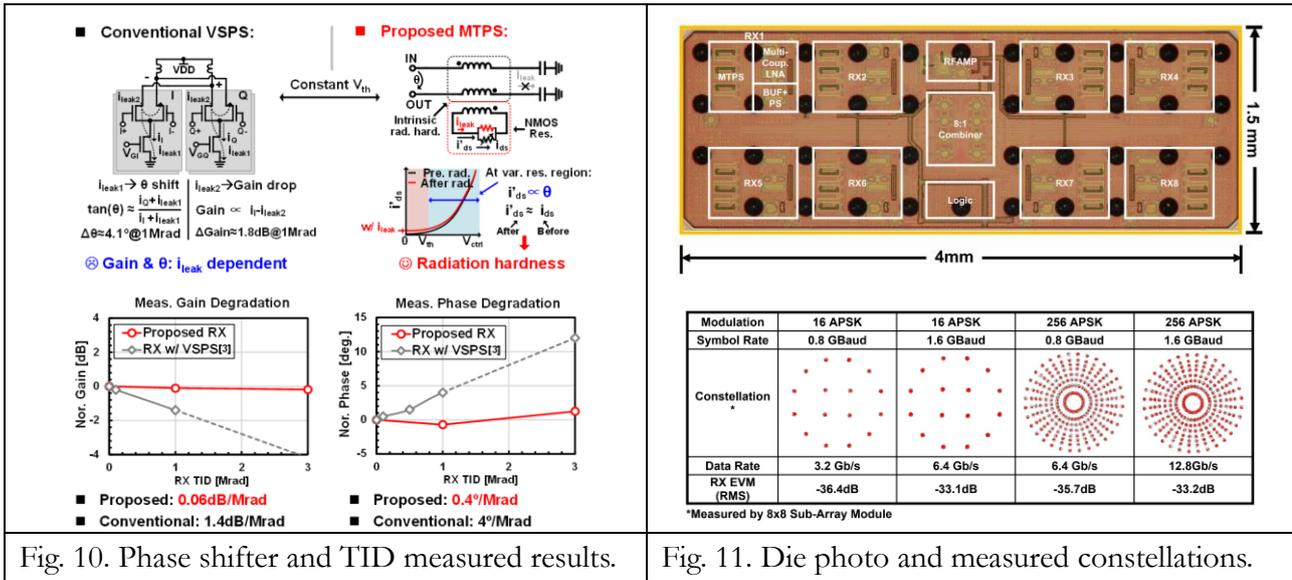
Fig. 10. Phase shifter and TID measured results.
