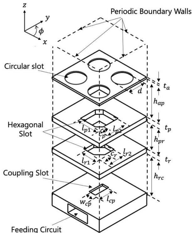
Fig. 1 Antenna structure
