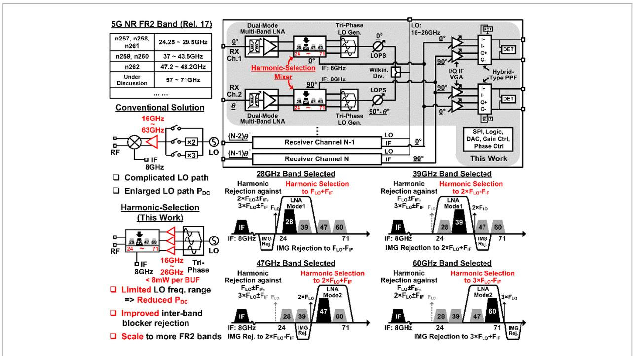
Fig. 5. Block diagram of proposed multi-band phased-array receiver.
