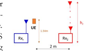
Fig. 1. Measurement Setup
