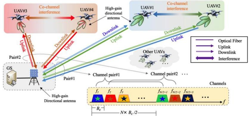
Fig. 5. Multi-UAV Full-duplex Communication System
