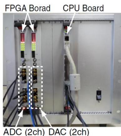
**Fig. 12. 60 GHz transceiver of OFDM experimental system**
