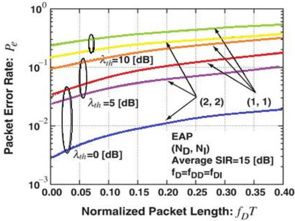
**Fig. 6** Packet error rate for the EAP condition:  $P_e$
