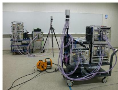
Fig. 1 Double directional channel measurement in  $24 \times 24$  MIMO configuration
