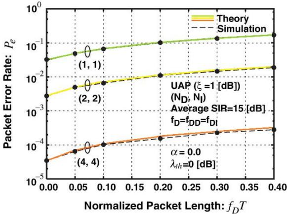
**Fig. 7** Packet error rate for the cellular system ( $\alpha = 0.0$ ) under the UAP condition ( $\xi = 1$  dB):  $P_e$
