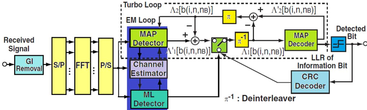
**Fig. 1. Structure of a suboptimal OFDM receiver**
