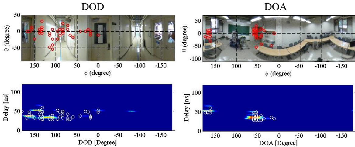
Fig. 2 Indoor double directional measurement example; results of beamforming and SAGE (space-alternating generalized expectation-maximization)
