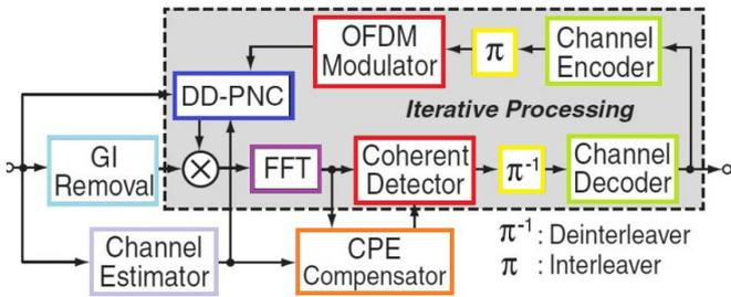
**Fig. 9. OFDM demodulation employing DD-PNC**
