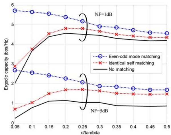
Fig. 15 Ergodic capacity as antenna distance
