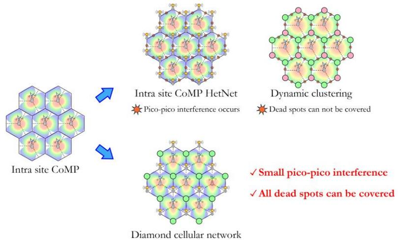
**Fig4. Conventional cellular network and Diamond cellular network**
