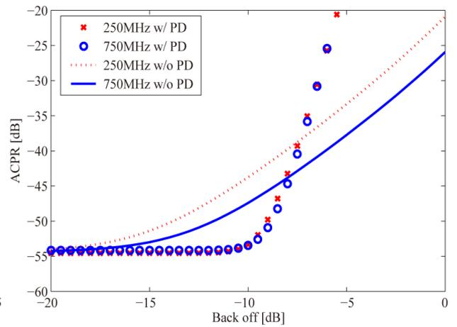
Fig.25 ACPR in dual-band OFDM system
