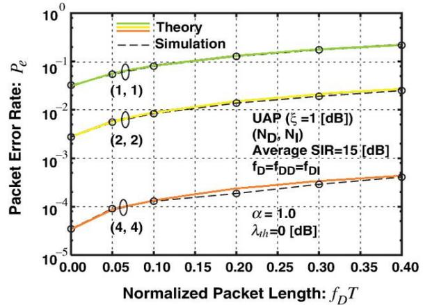
**Fig. 8** Packet error rate for the ad-hoc network ( $\alpha = 1.0$ ) under the UAP condition ( $\xi = 1$  dB):  $P_e$
