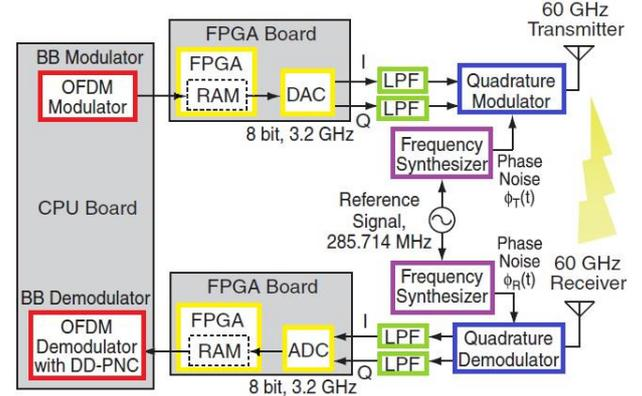
**Fig. 10. 60 GHz OFDM experimental system**
