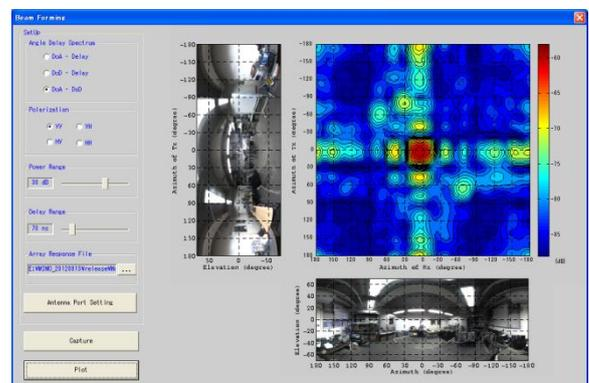
Fig. 5 The GUI of the in-situ validation tool. The measured data is analyzed and converted to angle-delay power spectrum that can be compared with the panorama pictures
