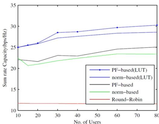
Fig. 16 System capacity vs. number of users
