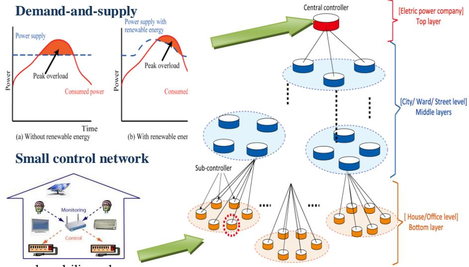
**Fig.27 Hierarchical Distributed Control Network**
