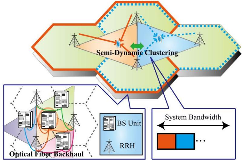
Fig. 1 Shared Remote Radio Head Architecture
