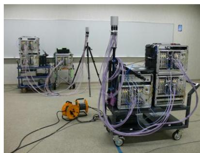
Fig. 1 Double directional channel measurement in  $24 \times 24$  MIMO configuration
