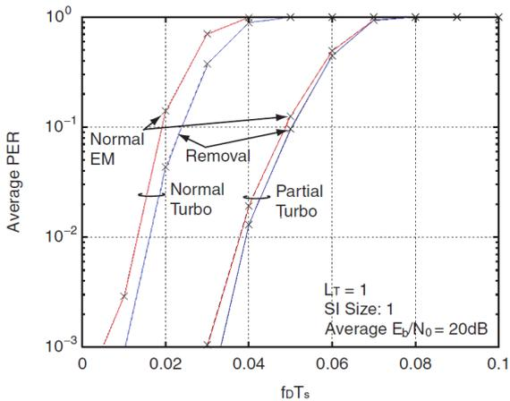
**Fig. 2. PER performance versus  $f_D T_s$  with  $L_T = 1$**
