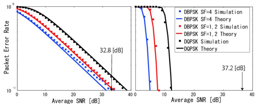
Fig. 21 Packet Error Rate (Left:  $m = 0.32$ , Right:  $m = 22.69$ )
