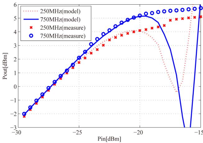
Fig. 24 Modeling for the nonlinear PA
