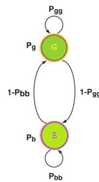
Fig. 5 Finite time-interval Markov model
