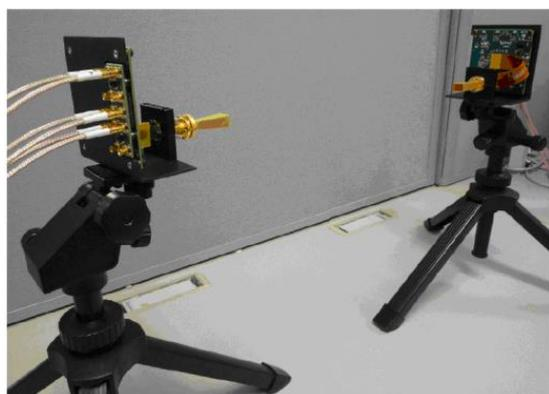
**Fig. 11. BB circuit of OFDM experimental system**
