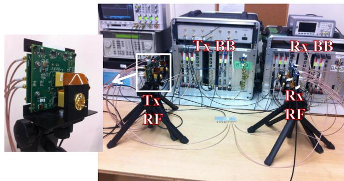
Fig. 6 60-GHz Millimeter-wave Channel Sounder
