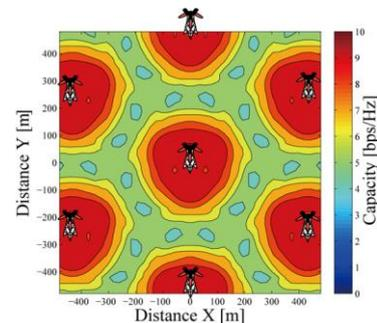
**Fig.7 BSC by optimal tilt angle**
