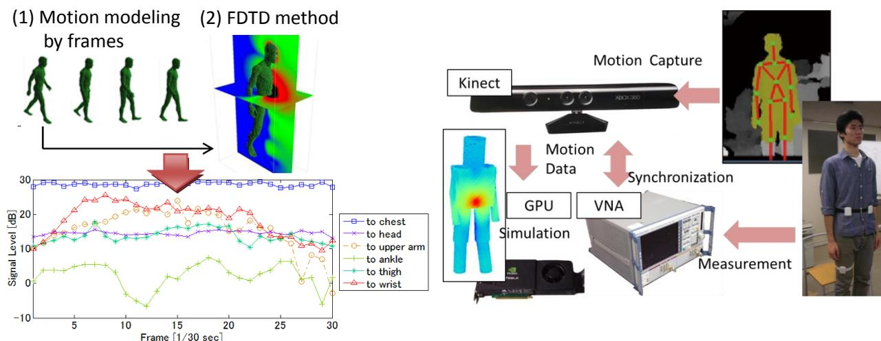
Fig. 13 (a) FDTD Simulation procedure and obtained result of link fluctuation (b) Integrated simulation and measurement environment using Kinect
