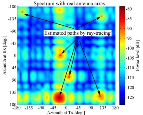
Fig. 7 Simulated double-directional angular power spectrum.
