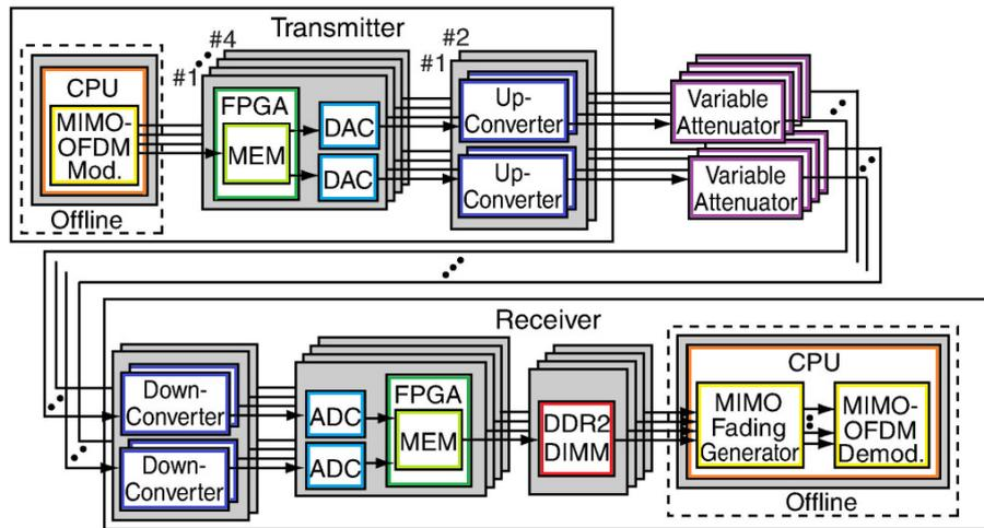
**Fig. 14. 11 GHz band 8x8 MIMO-OFDM experimental system**
