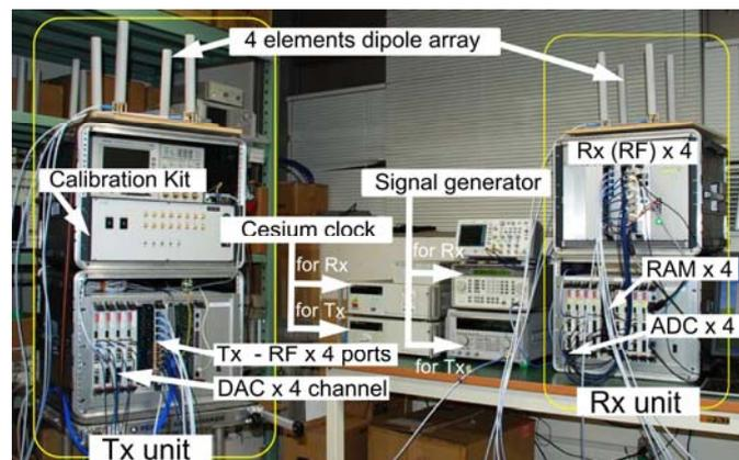
**Prototyping  $4 \times 4$  MIMO Channel Sounder**
