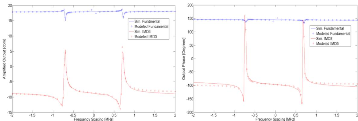
Figure1. Modeled Amplitude and Phase of Fundamental and IMD3
