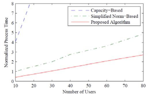
**Fig. 2** Normalized process time of the algorithms for multiuser BD 2 x 8 MIMO systems.
