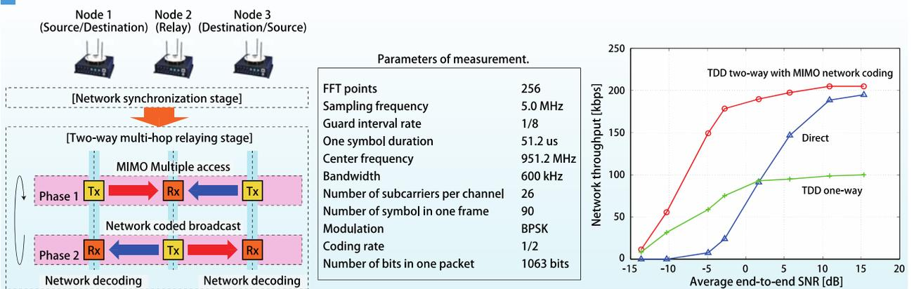
Fig. 3 Network throughput measurement of TDD two-way multi-hop relay network using MIMO network coding in an indoor environment.
