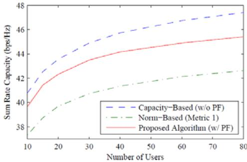
**Fig. 1** Average sum rate capacity for a multiuser 2 x 8 MIMO system with PF (SNR = 20 dB).
