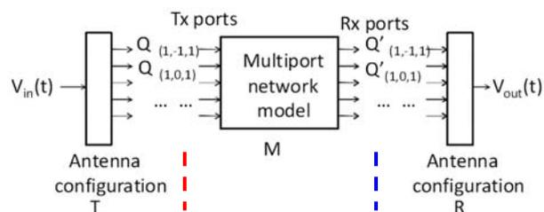
Equivalent circuit model of double-directional channel
