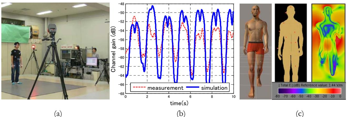
Research on BAN (a) measurement with motion capture (b) result of analytical simulation based on antenna motion (c) numerical simulation by Poser and XFDTD software
