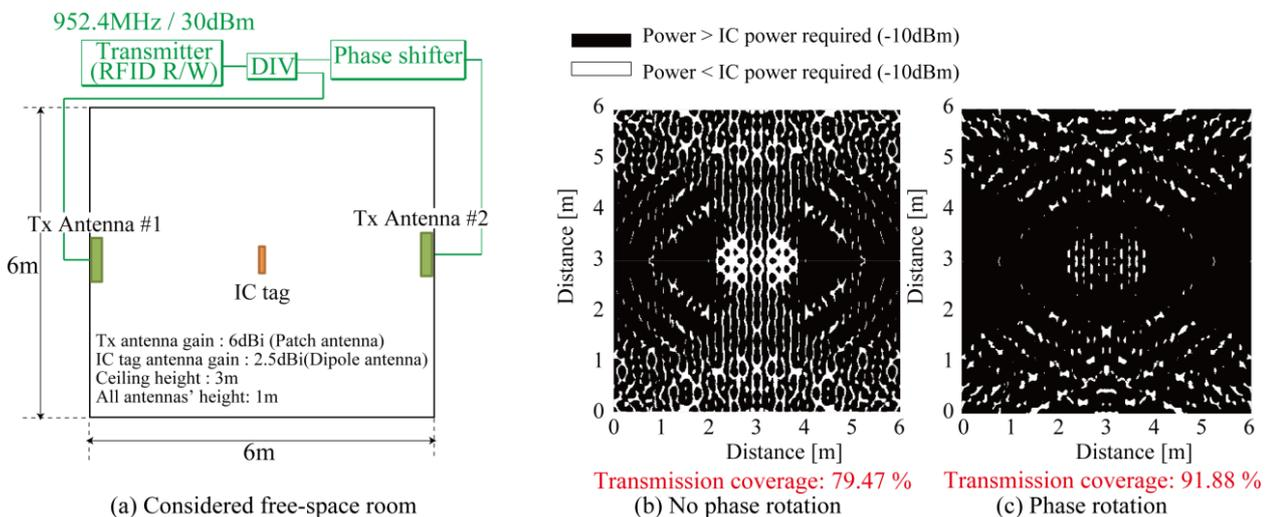
Fig. 2 Coverage of wireless energy transmission using multi-point
