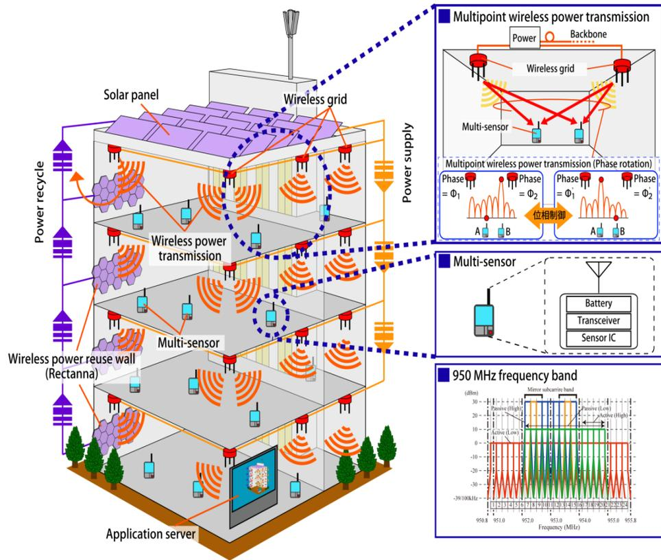
Fig. 1 Building control system with wireless grid
