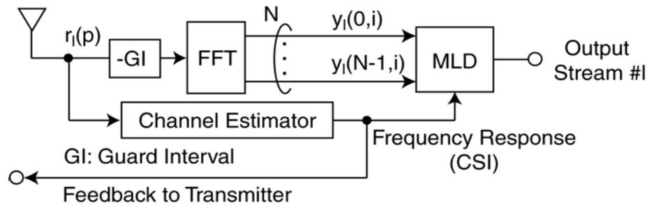
**Fig. 2 Receiver in downlink multiuser MIMO-OFDM**
