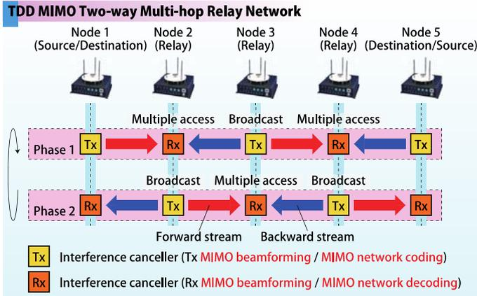
Fig. 1 TDD MIMO two-way multi-hop relay network.
