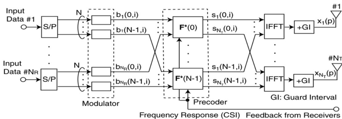
**Fig. 1 Transmitter in downlink multiuser MIMO-OFDM**
