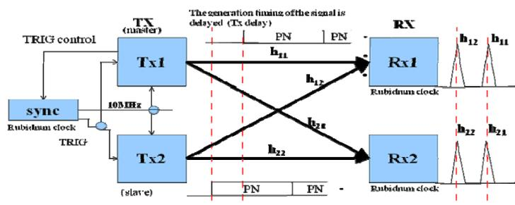
TDM MIMO channel sounding by using PN sequence
