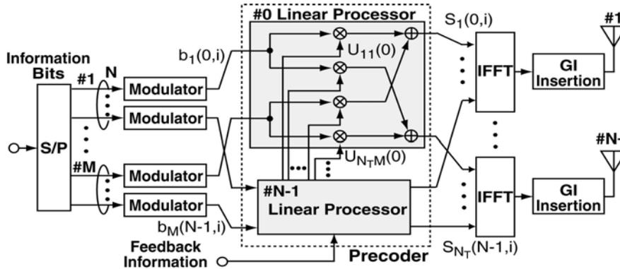
Fig. 8 Transmitter employing MBER precoding
