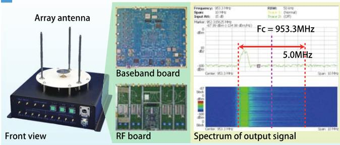
Fig. 2 Prototype hardware operating at 950MHz band.
