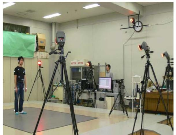
Fig. 9 Measurement of on-body channel fading with motion capture equipment.
