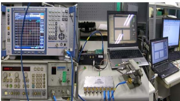
Fig.11 Spectrum sensing system setup
