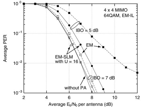
**Fig. 7 Average PER performances of EM-SLM with PA**
