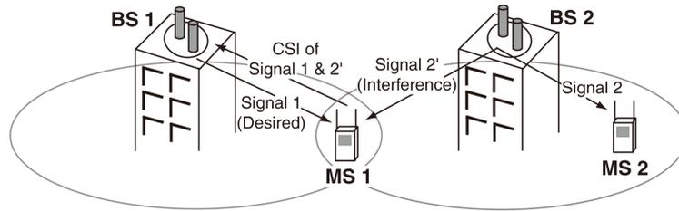
**Fig. 11 Downlink system in a multicell environment.**
