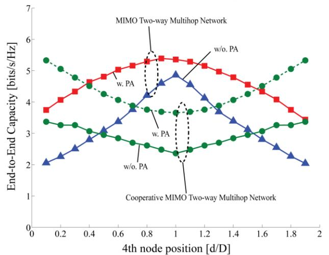
End-to-end capacity vs. central node position
