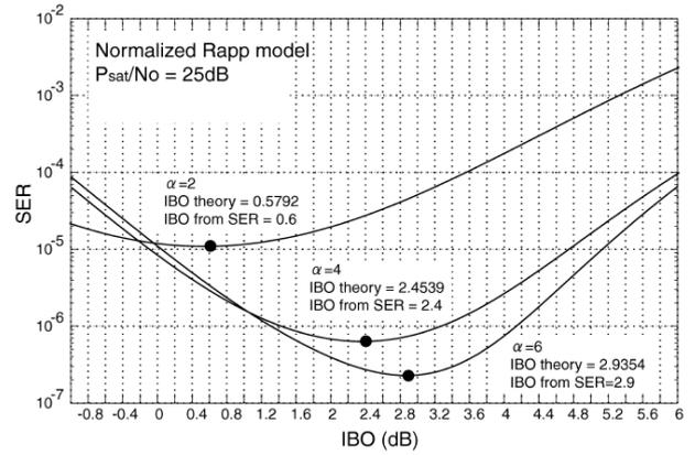
Normalized Rapp model: optimal IBO
