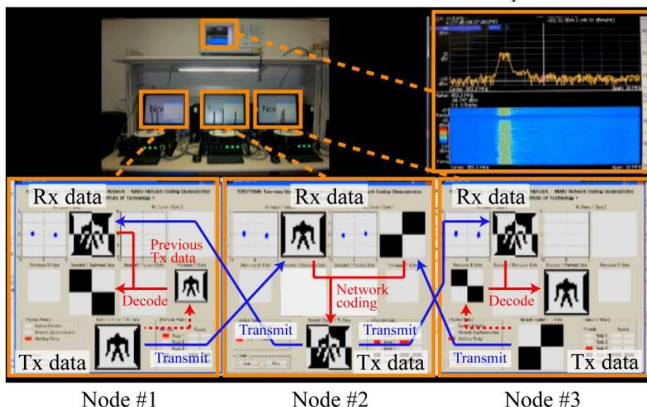
**MIMO two-way multi-hop relay network demonstrator with MIMO network coding using 950MHz band**
