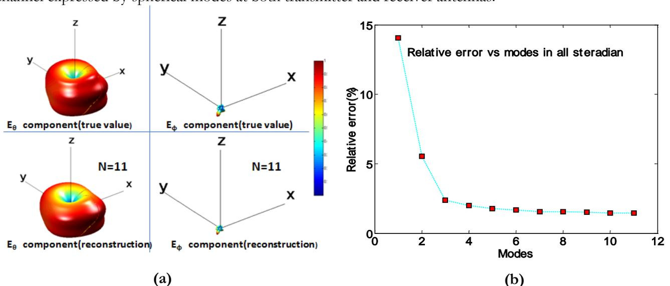
Fig.16 (a) Comparison the measured and reconstructed pattern at the number of a mode, (b) Relative Error VS N for measurement
