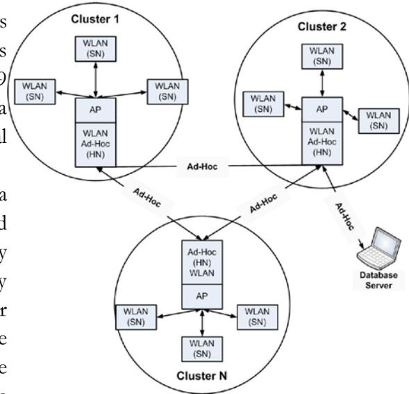
Fig.10 Cluster based Sensor Networks
