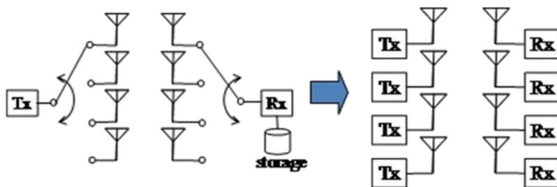
Fig.6 MIMO Channel Sounder Structure
