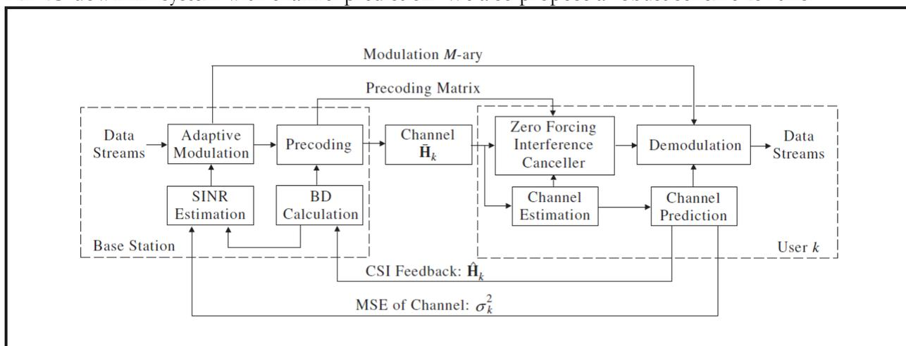
System design for robust multiuser block-diagonalization
