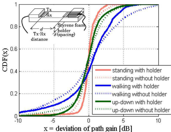
Fig. 8 Effect of antenna rotation was decomposed by two-antenna holder.
