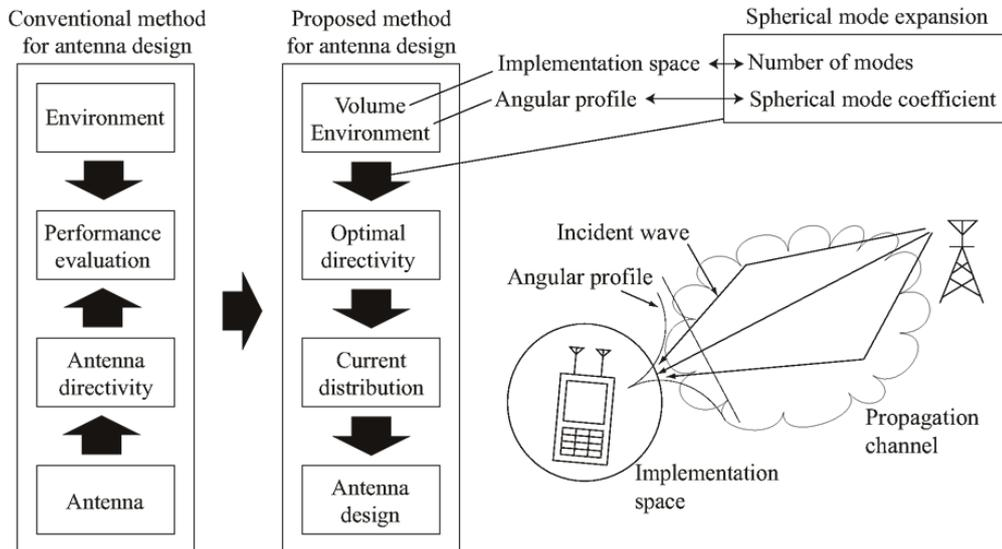
Spherical Mode Expansion – based diversity antenna design
