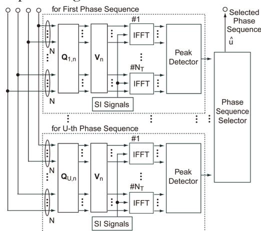
Fig. 4 Phase sequence controller for EM-SLM
