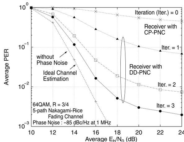
**Fig. 2 Average PER performance with 64QAM**
