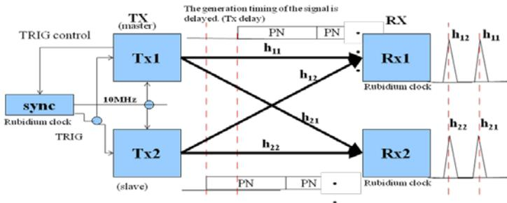
Fig.17 TDM MIMO channel sounder using PN sequence
