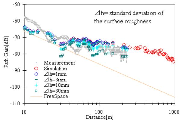
Fig.15 Path gain results with the rough surface.
