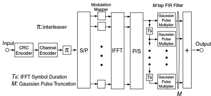
**Fig. 8 GS-OFDM transmitter**
