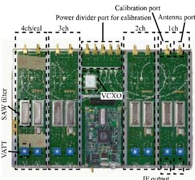
Fig.6 RF board of cognitive MIMO mesh relay node
