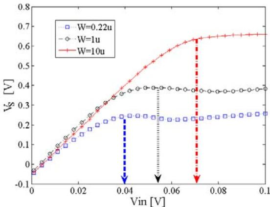
Fig.6 Saturation vs Gate-width performance
