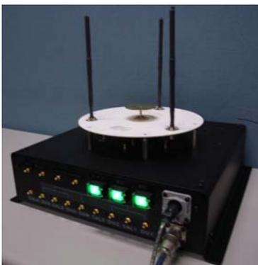
Fig.4 Overview of cognitive MIMO mesh relay node.
