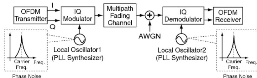
**Fig. 12 Phase noises in OFDM transmission**
