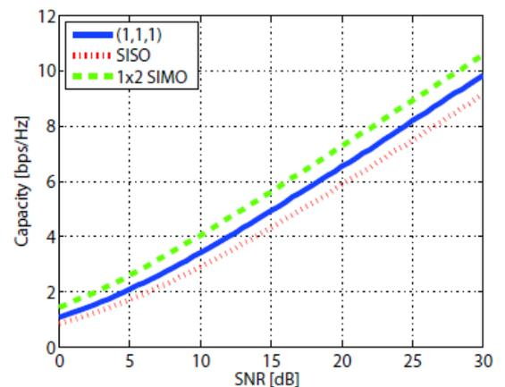
Fig. 3 Capacity using a parasitic antenna element
