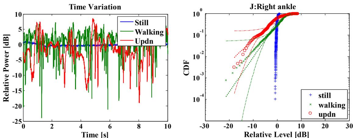
Figure: (a) Path gain variation in a movement scenario and (b) cumulative distribution of the path gain (dashed line : log-normal distribution fitting and dotted line: Weibull distribution fitting)
