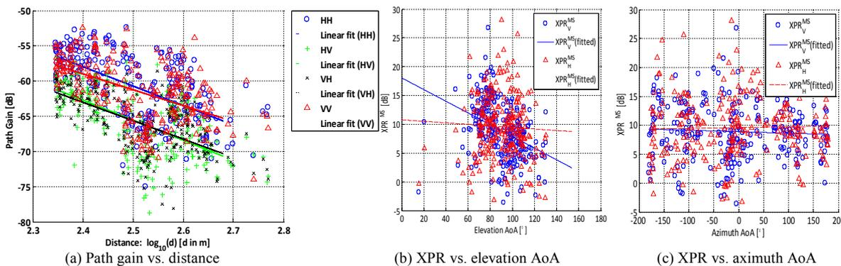
Examples of the polarization characteristics (Path gain, XPR at MS)
