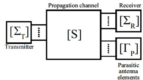
Fig.1 Tandem of channel, transmitter, receiver and parasitic antenna elements
