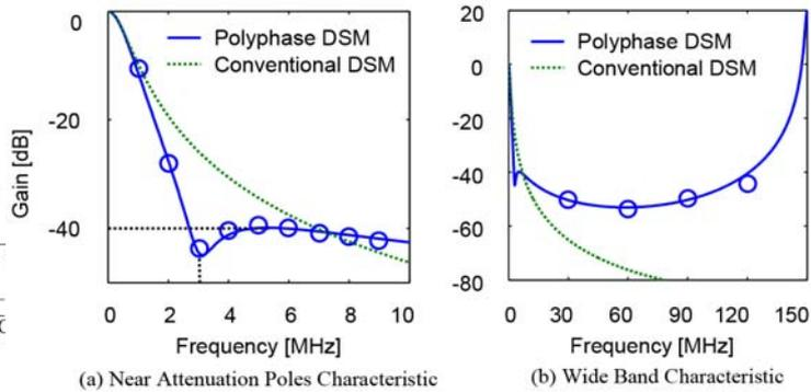
Fig.5 Frequency Characteristics
