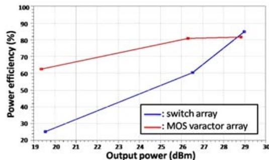
Fig2 Comparison of power efficiency
