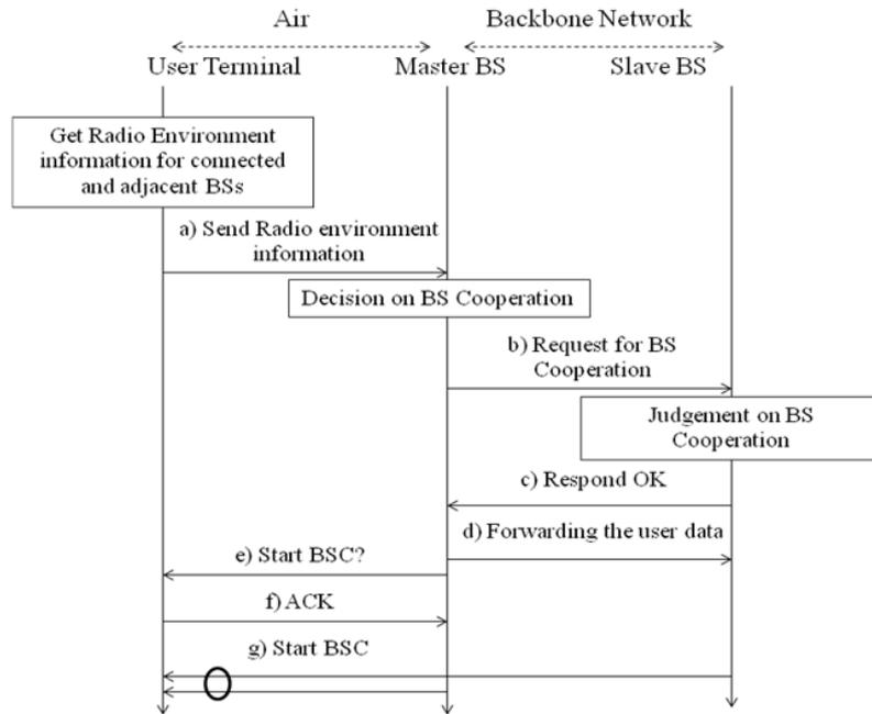
Fig.3 Fractional Base Station Cooperation Procedure
