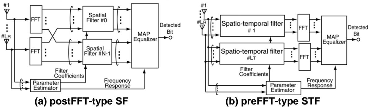
**Fig. 2 Two conventional methods for implementing SF**
