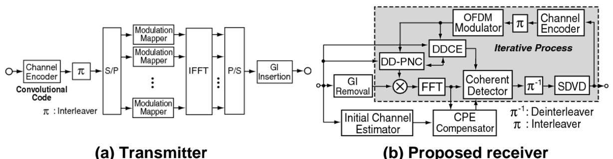
**Fig. 13 OFDM system model**
