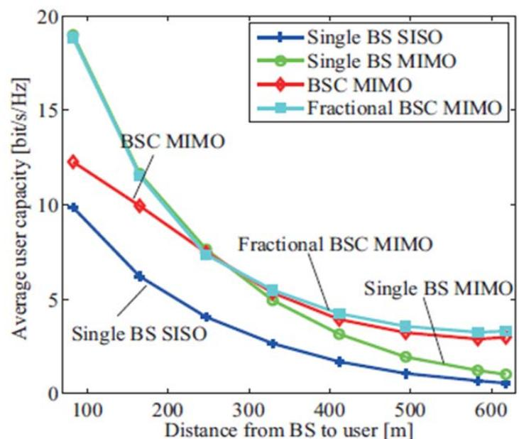
Fig.2 User Capacity vs. Distance
