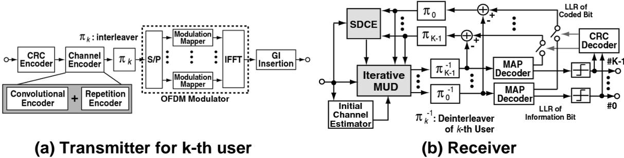
**Fig. 5 Proposed uplink MC-IDMA system**
