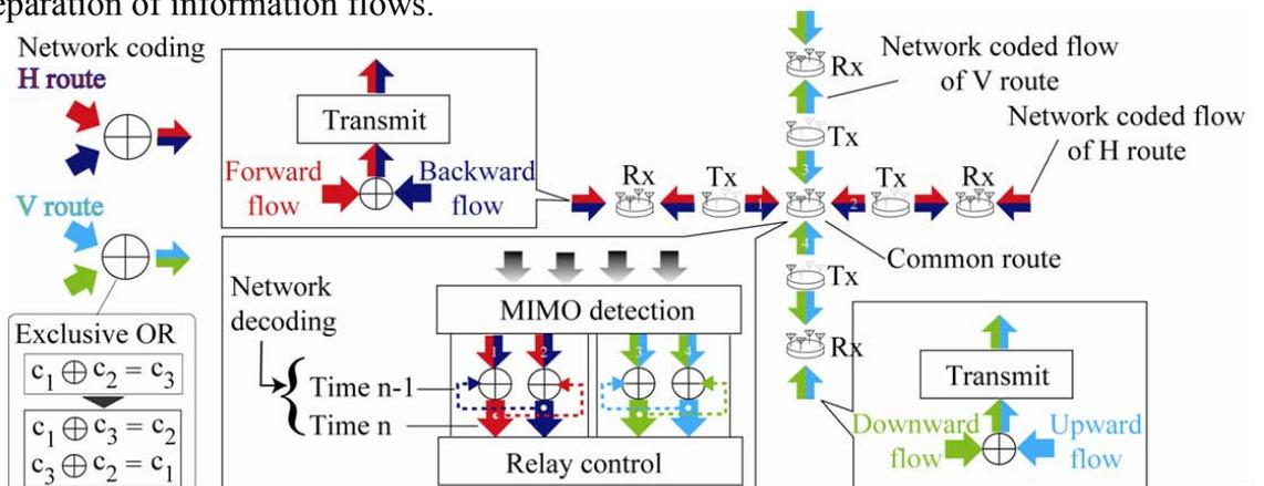
Fig.2 Algorithm of 2D MIMO network coding
