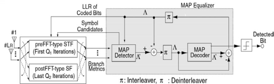
**Fig. 3 Proposed MAP receiver with preFFT-type STF / postFFT-type SF switch**
