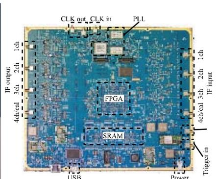
Fig.5 Baseband board of cognitive MIMO mesh relay node
