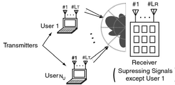
**Fig. 1 System model of uplink communication with SF**
