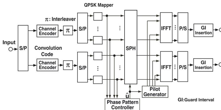
**Fig.4 Block diagram of the transmitter employing SPH-SLM**
