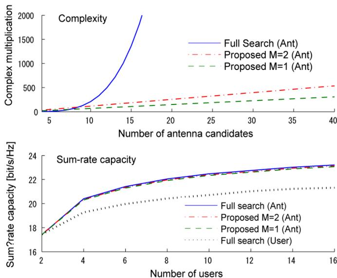
To achieve the maximum capacity in multi-user MIMO systems, antennas configuration and user selection are performed simultaneously. The proposed algorithm can also be considered as an extended application of the  $M$ -algorithm proposed in QRM-MLD algorithm.
