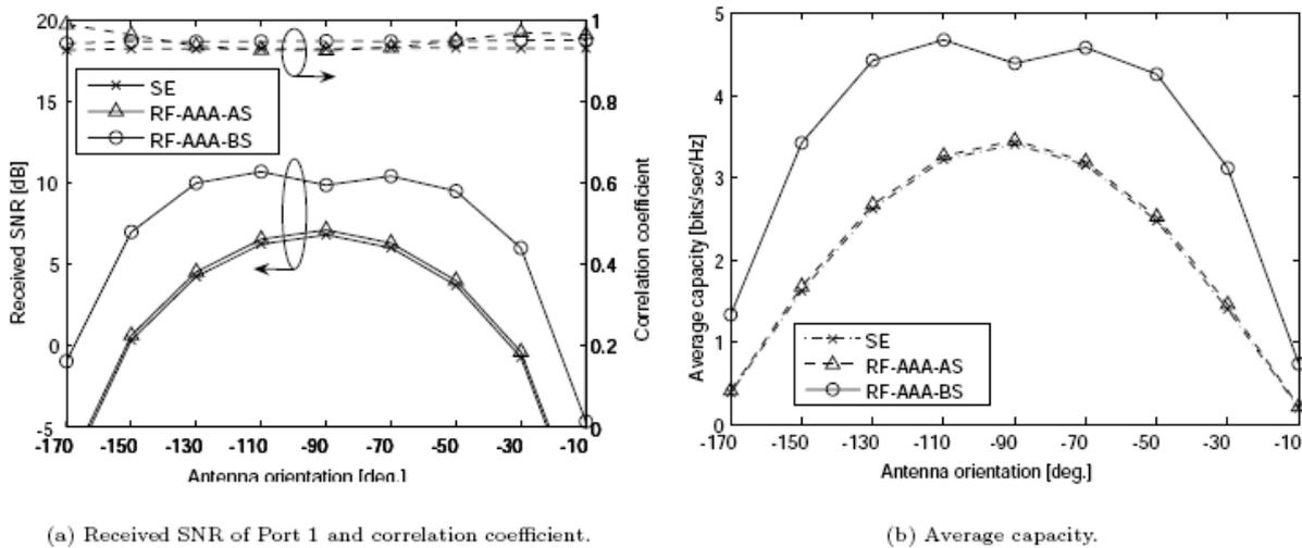
Fig. 1 Transmission characteristics when the antenna orientations are changed in the LOS environment.
