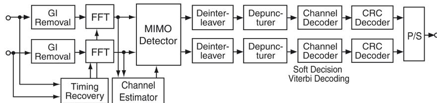
Fig.1 Block diagram of the receiver module
