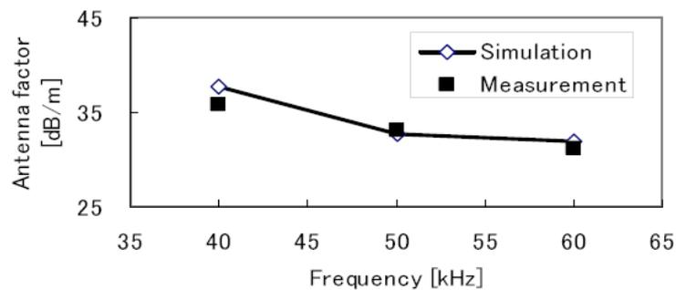
Fig. 3 Antenna Factor of the MCLA
