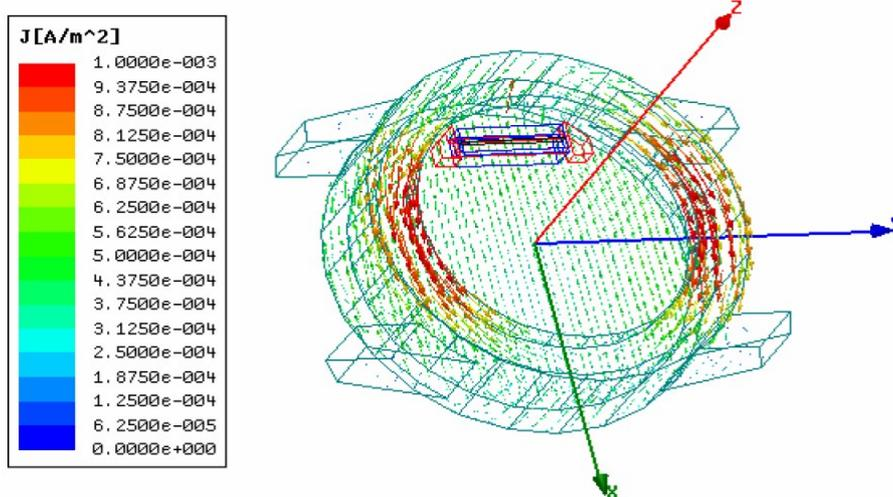
Fig. 4 Current density generated in a metal case
