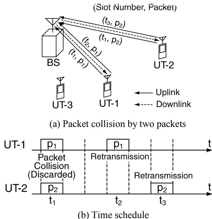
Fig.1 Mobile radio packet system with random access protocol
