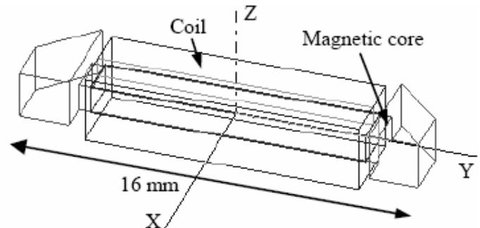
Fig. 2 Simulation model of the MCLA
