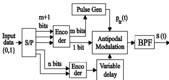
This modulation scheme, PMM(n,m) will increase the total data rate of system which depends on both the number of pulse positions ( $N = 2^n$ ) and the number of different pulses ( $M=2^m$ ) that have been used in the system. Then, PMM(n,m) system can be transmitted  $n+m+1$  data bits per frame that is  $n+m+1$  times when compared to the conventional TR-UWB system.
