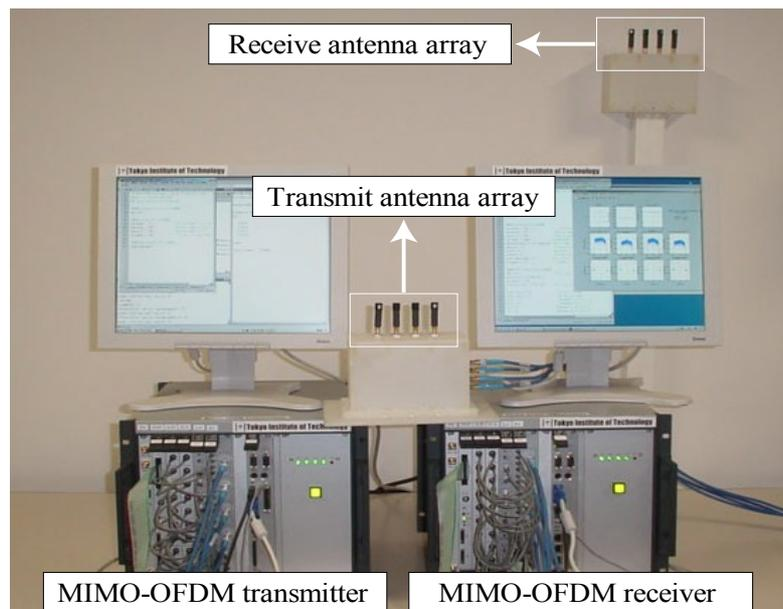
Fig1: The exterior of system
