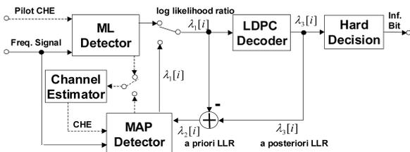
**Fig.4 block diagram of MAP receiver**
