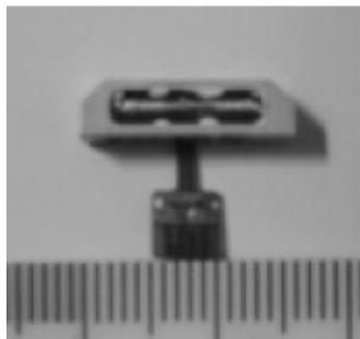
Fig. 1 The MCLA used in radio controlled watches
